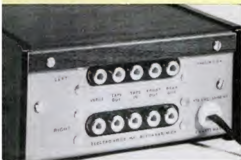
SMALL ELECTRO-VOICE DECODER , shown on top of receiver above, provides four-channel output from two- or four-channel sources, is priced at $59.95. Diagram on facing page shows hookup requiring second stereo amplifier as well as existing one. Photo below shows various connections on back of decoder
